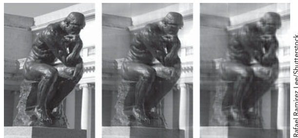
Image reproduced from 100% of the data in Fourier space, image reproduced from 1% of the data, and image reproduced from 0.006% of the data
